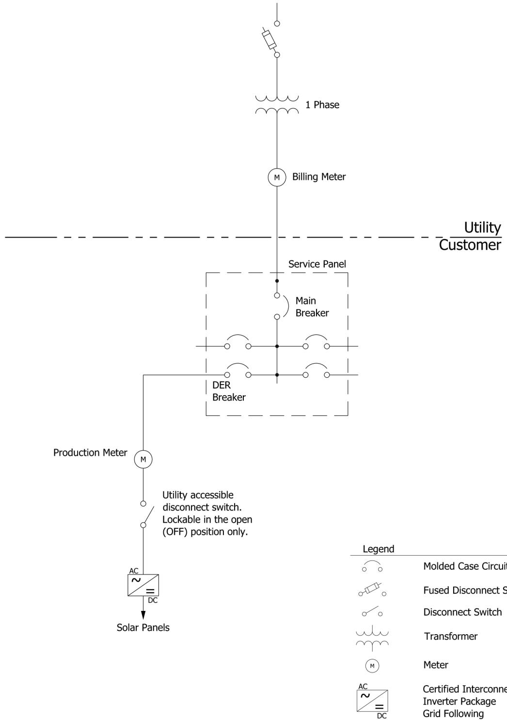
Sample One-Line Diagram for Certified Inverter Package Installations
