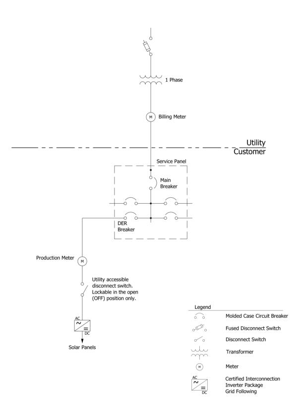
Sample One-Line Diagram for Certified Inverter Package Installations Less than 20kW
